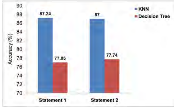
Fig. 4 The performance of K-NN and decision tree classifiers for the two statements “Kids are talking by the door” and “Dogs are sitting by the door” speech
