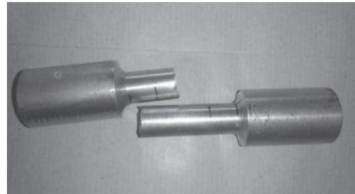
Tensile specimen after fracture
