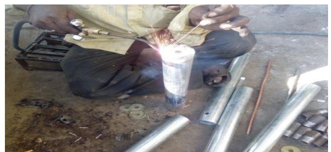
Figure 5 welding of washers
