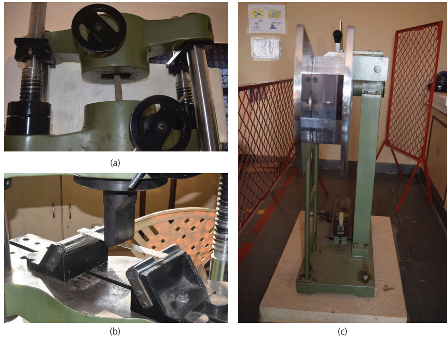
Figure 2. Testing of samples with fixture for (a) tensile loading, (b) flexural loading and (c) impact loading
