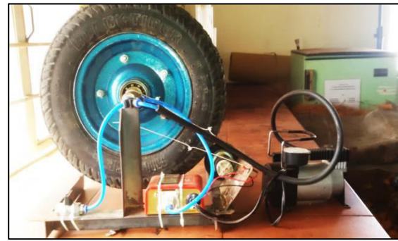
Fig 5 Model of running wheel air pressure monitoring system
