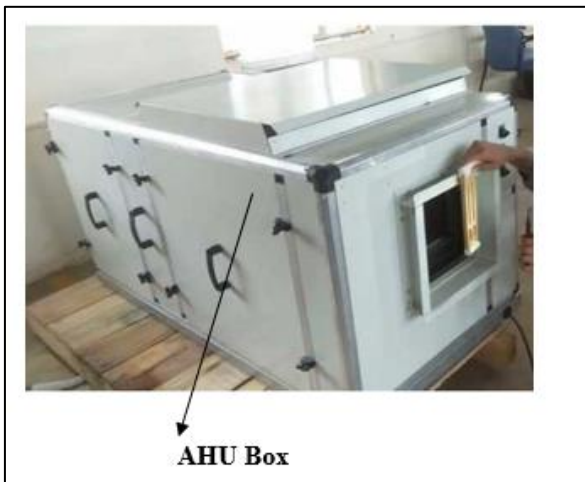
Fig. 13: Working model of an Evaporative Cooling System
