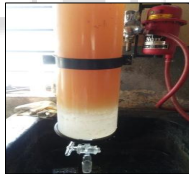
Washing of biodiesel with water and Drying.
