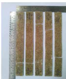
Fig. 6 Fractured Tensile test specimens.
