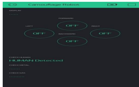
Working of PIR Sensor on Blynk Application
